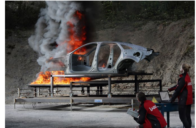
Fire test based on ECE R 100
