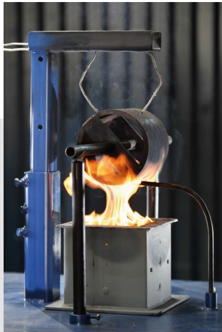
Fire test based on DIN EN 45545
