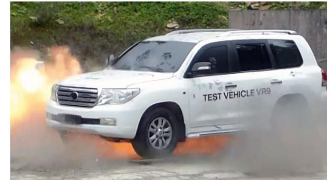
Blast test on a protected vehicle
