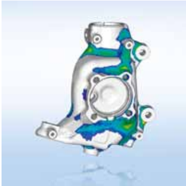
Above: Fatigue life assessment of a swivel bearing
