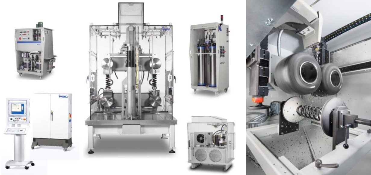
Figure 2: IABG resonance spring testing machine and grit impact simulator
