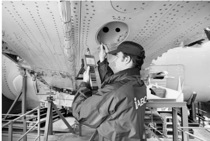
Figure 5: Eddy current inspection on the A320 NEF2 wing
