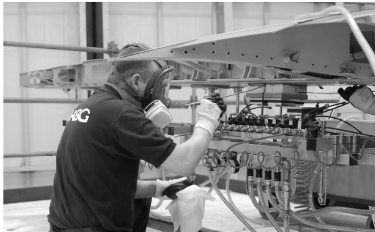
Figure 3: Pad Bonding at the A320 NEF test specimen
