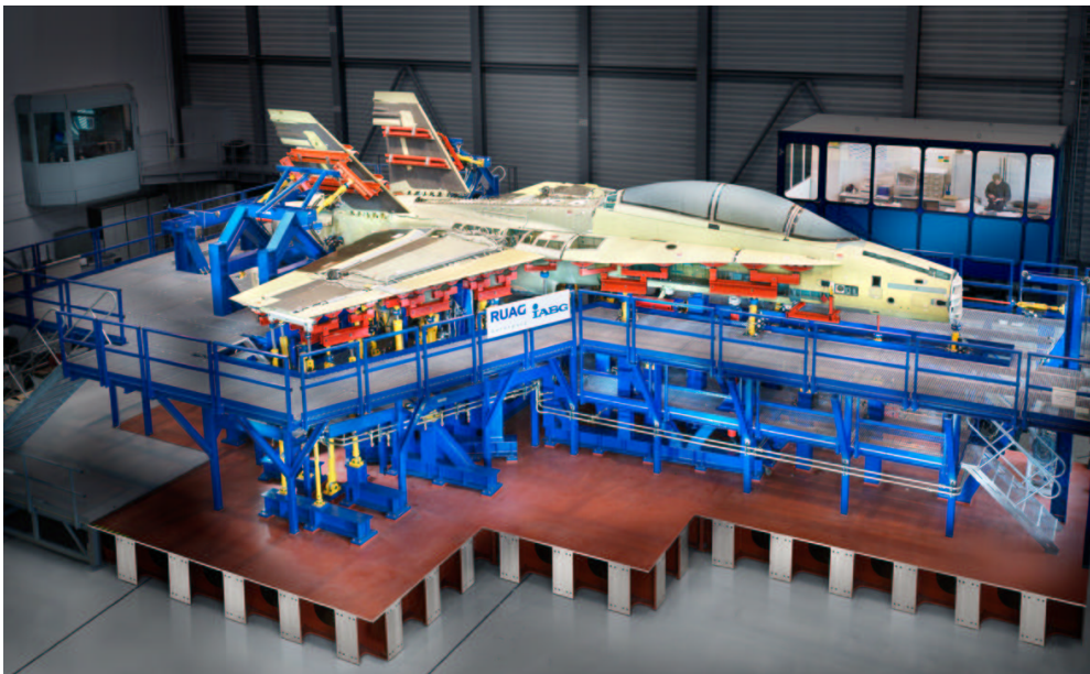
FIGURE 10 Complete test set-up for the Swiss F/A-18
