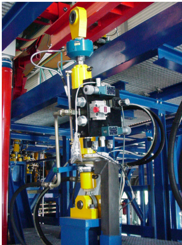
FIGURE 8 Complete assembly of hydraulic jack (FFZ2) at the front fuselage with manifold block, valves, load cell and bearings
