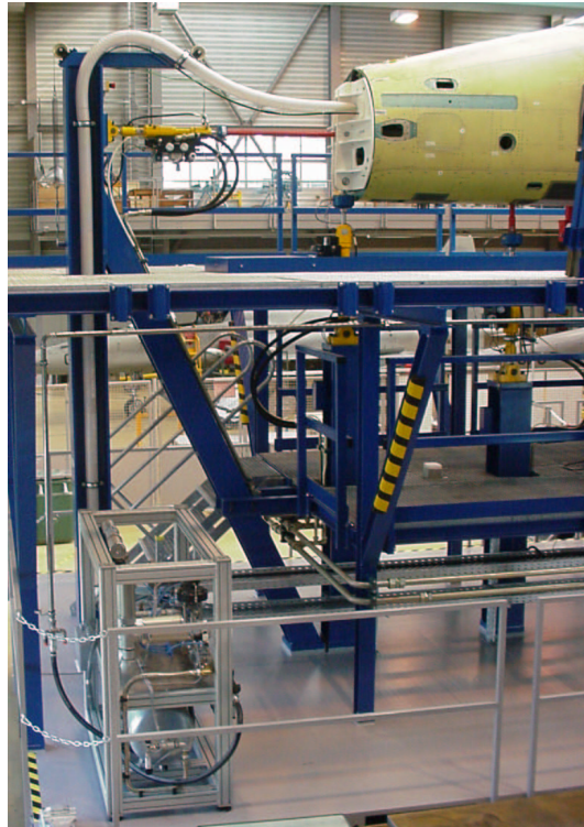
FIGURE 10 Complete test set-up for the Swiss F/A-18
