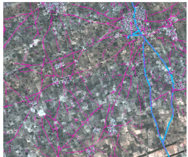
Fig. 4. Exemplary Planet Dove satellite image showing a region in Nigeria with a spatial resolution of 3 m. The corresponding OpenStreetMap data is illustrated in blue. Our prediction is shown in pink, given an impression of how many roads truly exist in this region.
