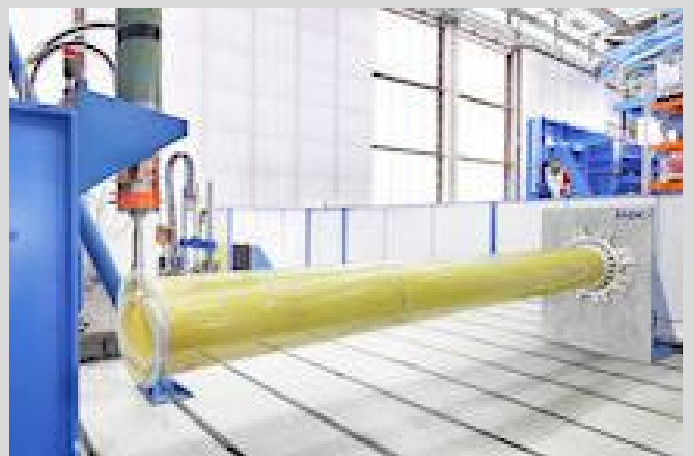
Bending test of an isolator on HYDRA test facility
