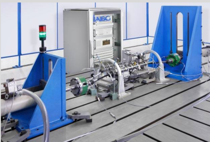
Test of a steering system on HYDRA test facility
