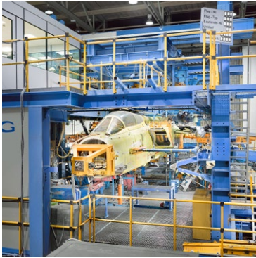
Major Airframe Fatigue Test on PA-200 Tornado
