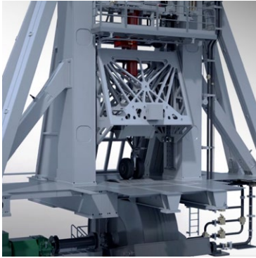
Chassis drum test rig for chassis analysis, validation and HIL simulation
