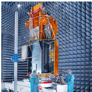
CryoSat spacecraft during EMC measurements
