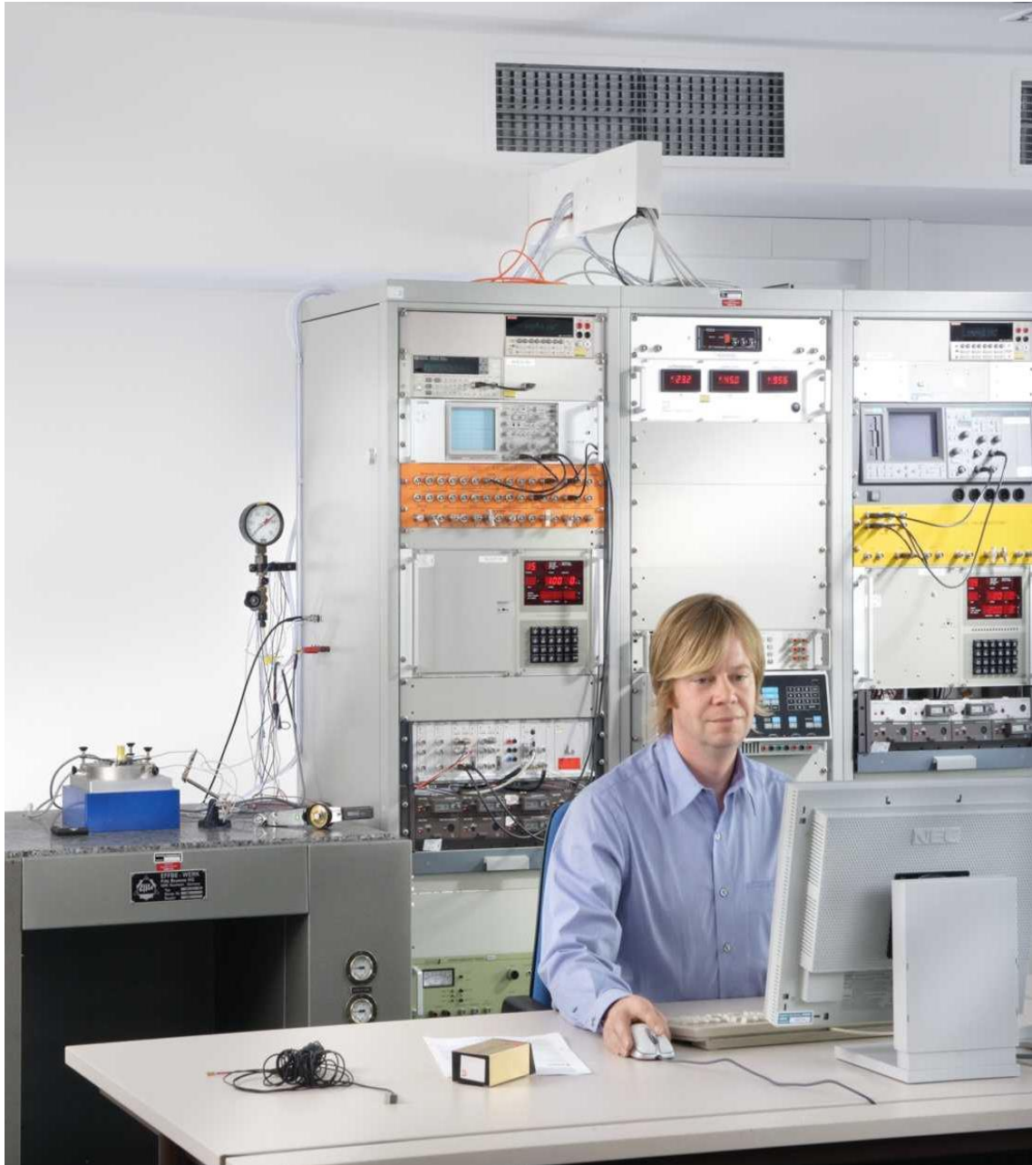
Sinusoidal Calibration of an Accelerometer
