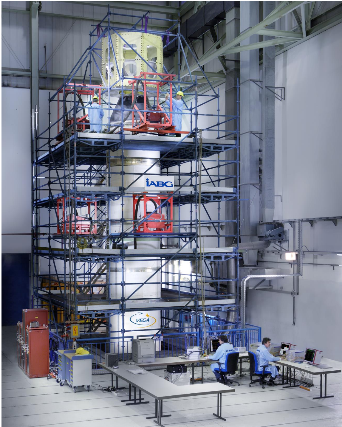
Modal Survey Test on VEGA Launcher
