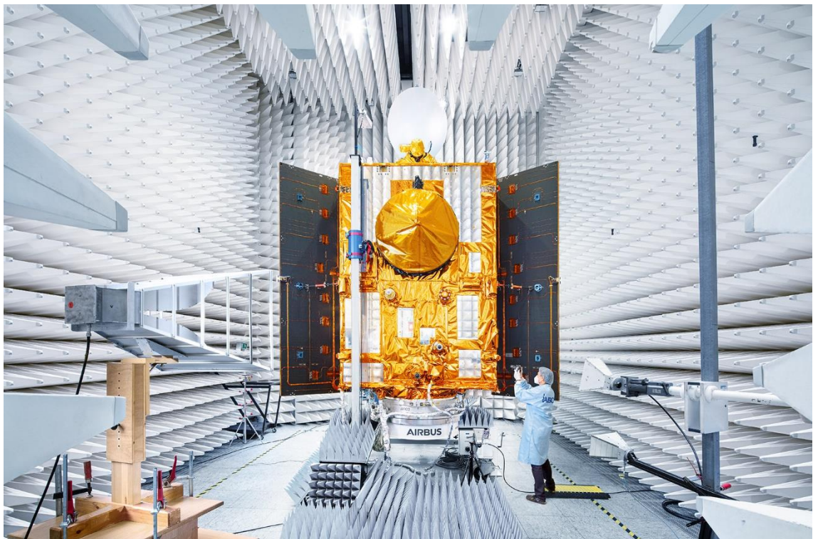
EMC Test on Sentinel 6 SAT-B S/C
