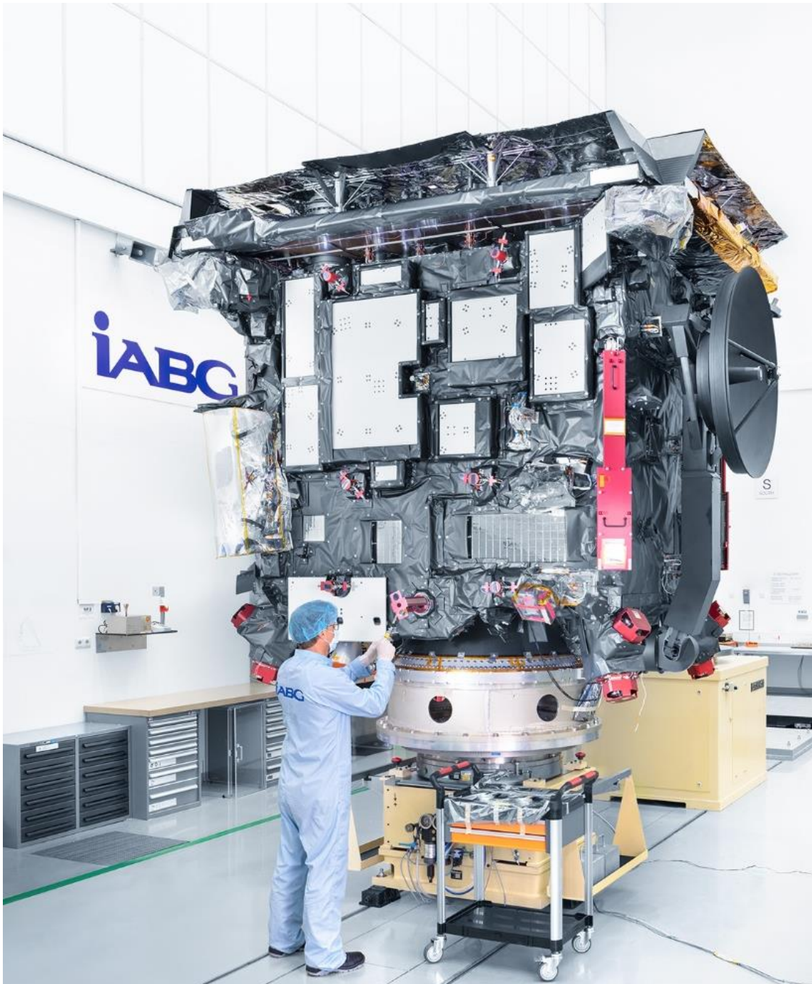
SOLAR ORBITER on the Mass Property Measurement Device ESA Mission with Airbus DS UK as prime
