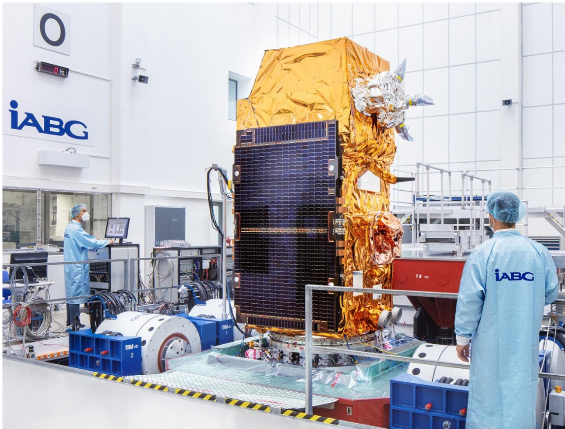
500 kN Multi-Shaker System with SENTINEL 2C S/C
