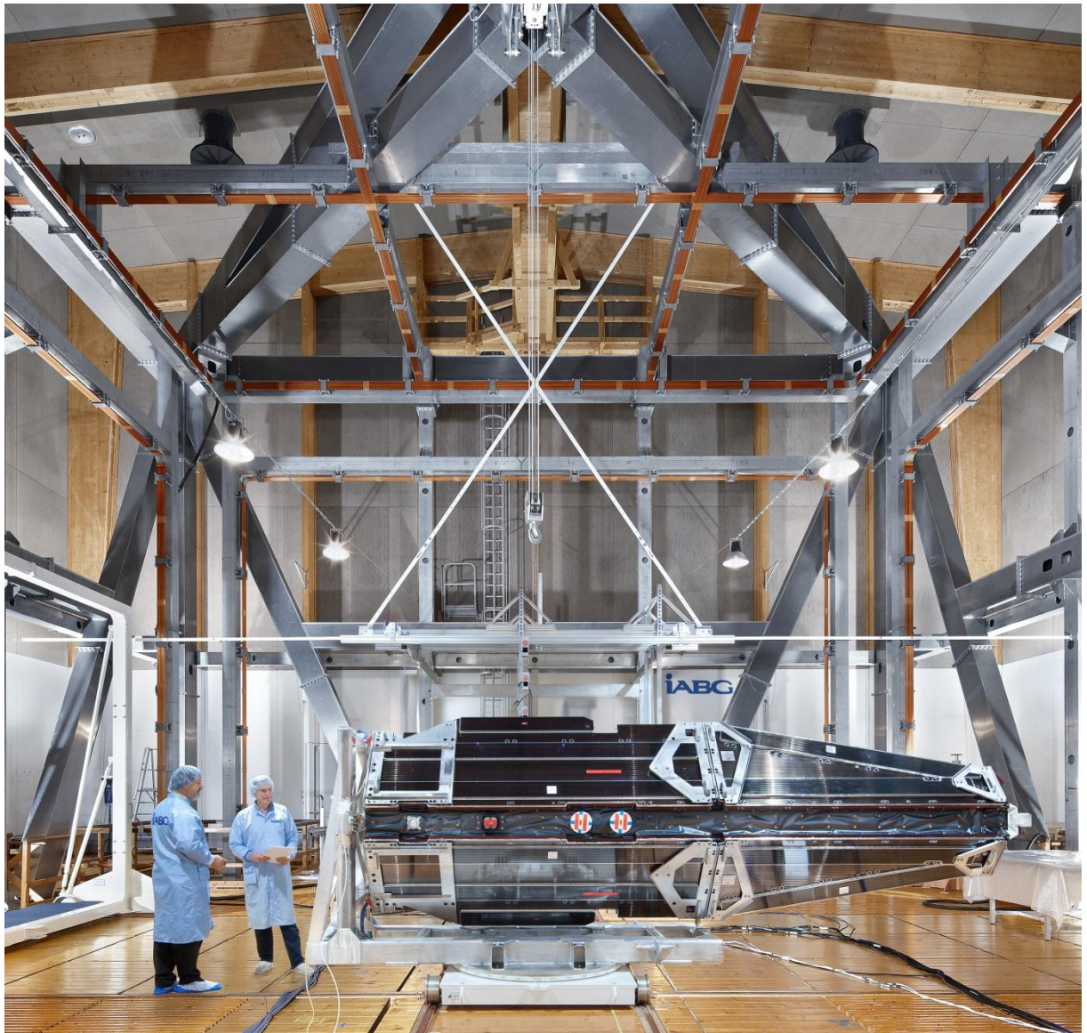
SWARM S/C during a magnetic test
