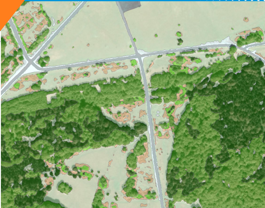
A subsection of the eCognition classification. IABG integrated LiDAR-derived DEMs, optical satellite imagery, aerial photos and other data into eCognition to distinguish Blackthorn from other vegetative types.
