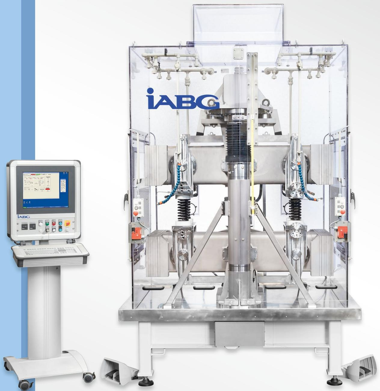
Resonance spring test stand with corrosion installation (optional with climatic simulation)
