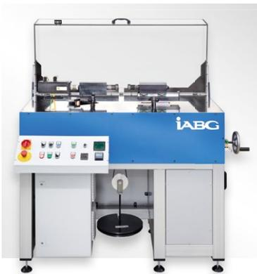
Test benches for fatigue testing of bogies
