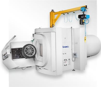
Wheel testing on the highspeed external drum test bench
