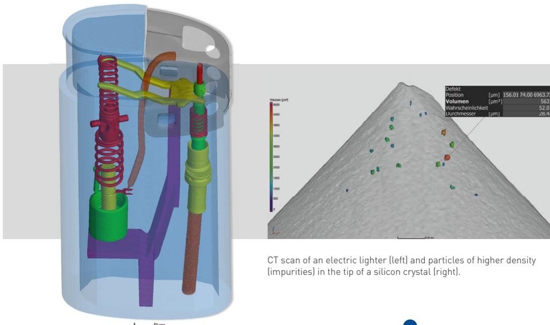
CT scan of an electric lighter (left) and particles of higher density (impurities) in the tip of a silicon crystal (right).
