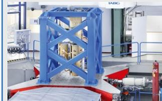
Multi-axis vibration and seismic testing
