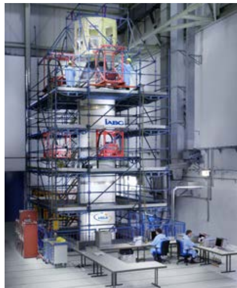
Modal survey test on the VEGA launcher
