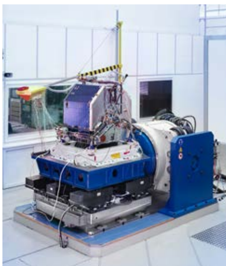
Philae on the 200 kN shaker
