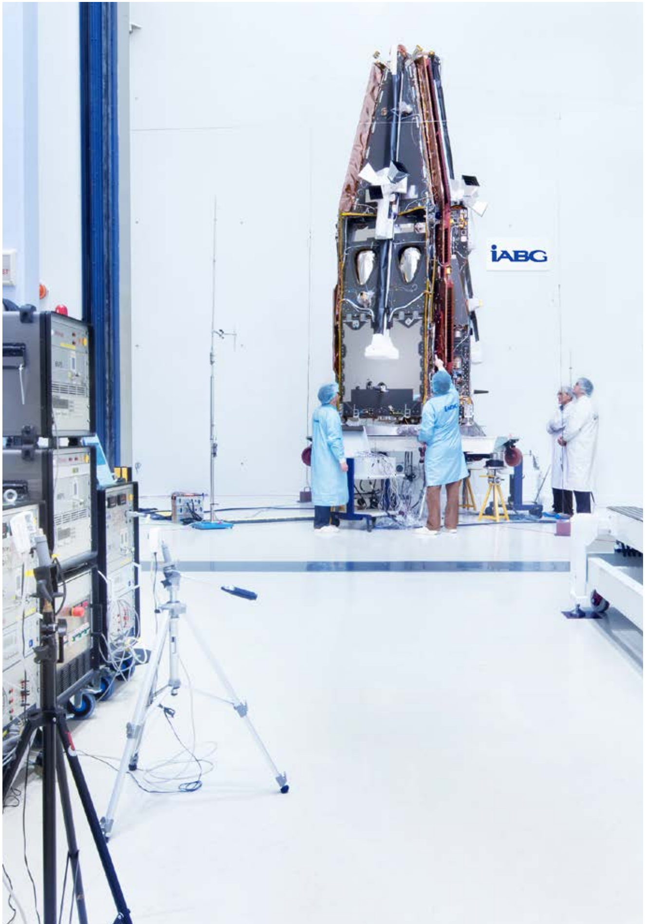
Acoustic noise test on Swarm satellites in stack configuration
