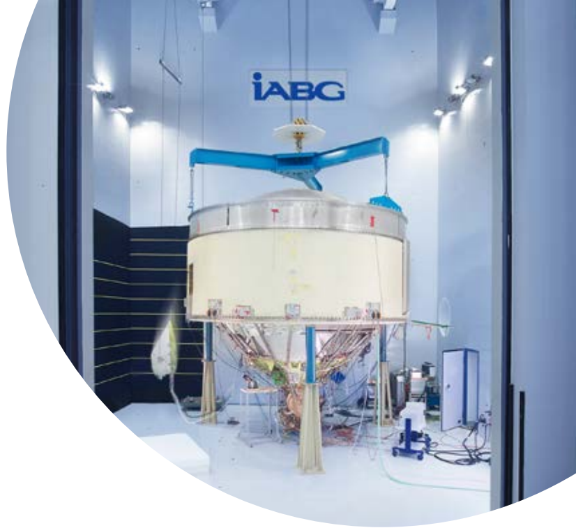
Separation shock test on ARIANE 5 ESC-A upper stage
