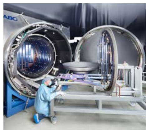
Thermal Vacuum Facility 2,5 m-He TVA including high temperature subsystem with ESA's Solar Orbiter antenna reflector built by Airbus Defence and Space
