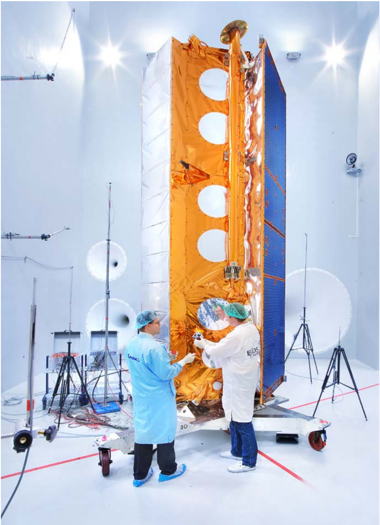
TerraSAR-X spacecraft during acoustic noise test
