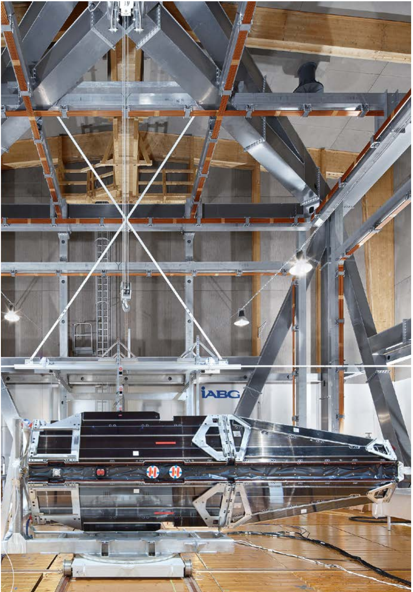
Swarm satellite in the magnetic test facility MFSA
