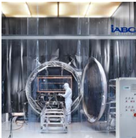
Cryogenic test facility 2.5 m He TVA with ISO 5 tent
