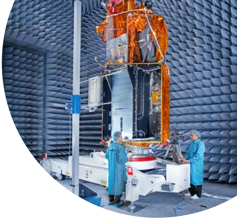
CryoSat spacecraft during EMC measurements
