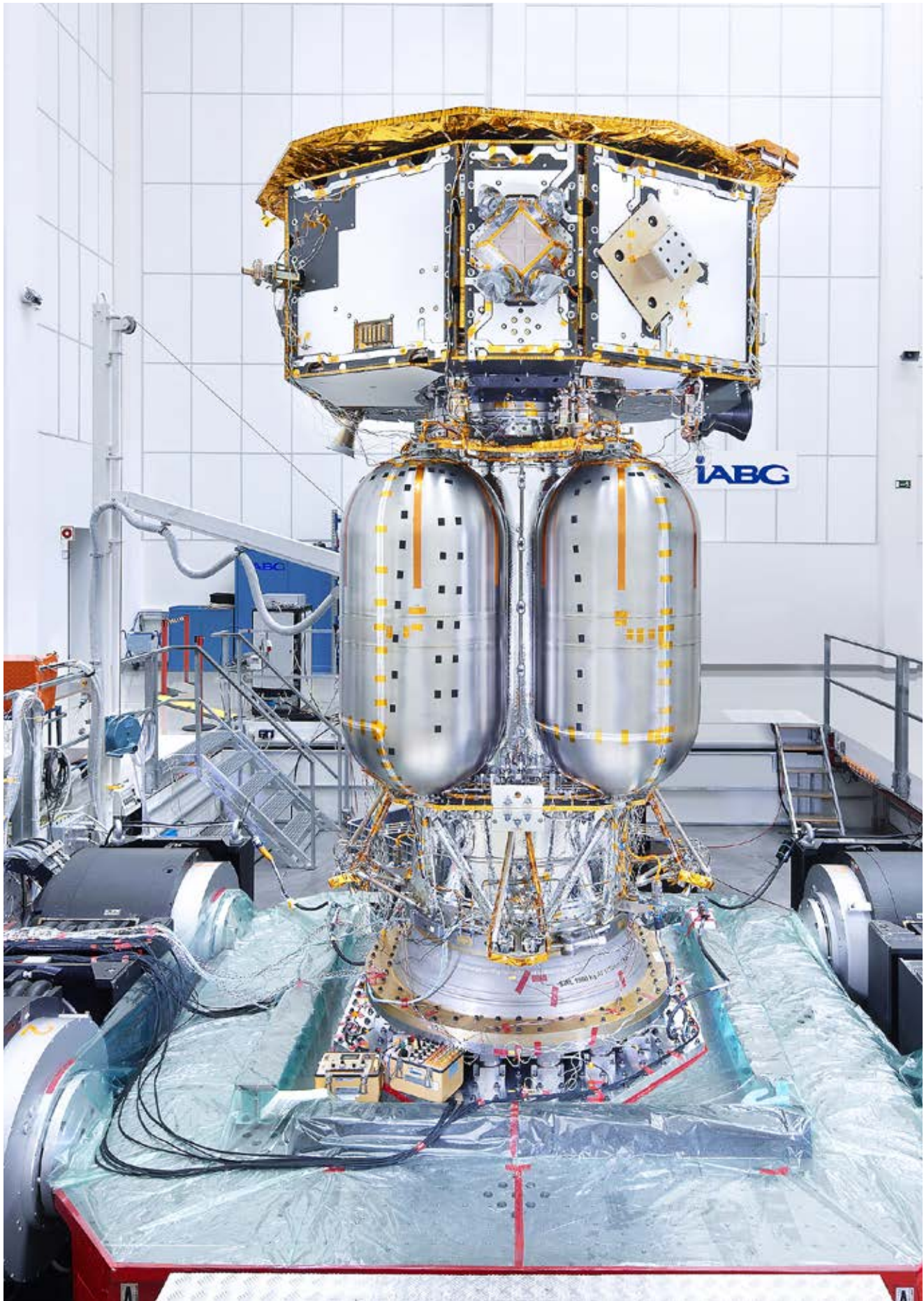
LISA Pathfinder LCM satellite on a 320 kN multi-shaker system
