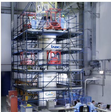
Modal survey test on VEGA launcher
