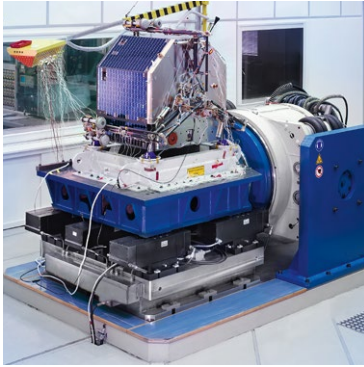
Philae on the 200 kN shaker
