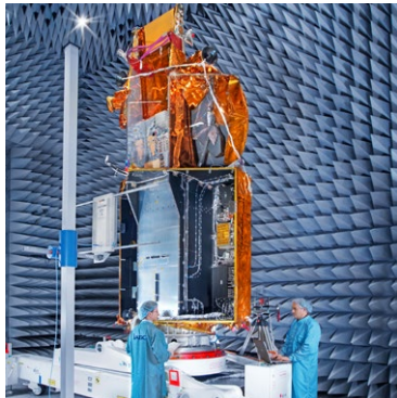
CryoSat spacecraft during EMC measurements
