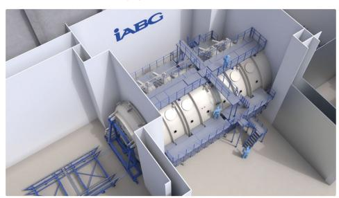
The TV Chamber is situated on the hall floor and spans the sprung mass of the Optical Bench Installation without any contact.
