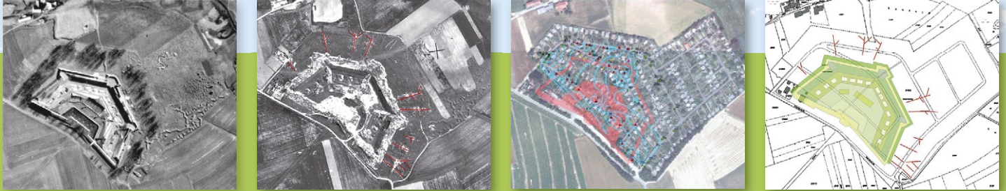
From a historical aerial photograph to the layout plan of a potential contamination site.
